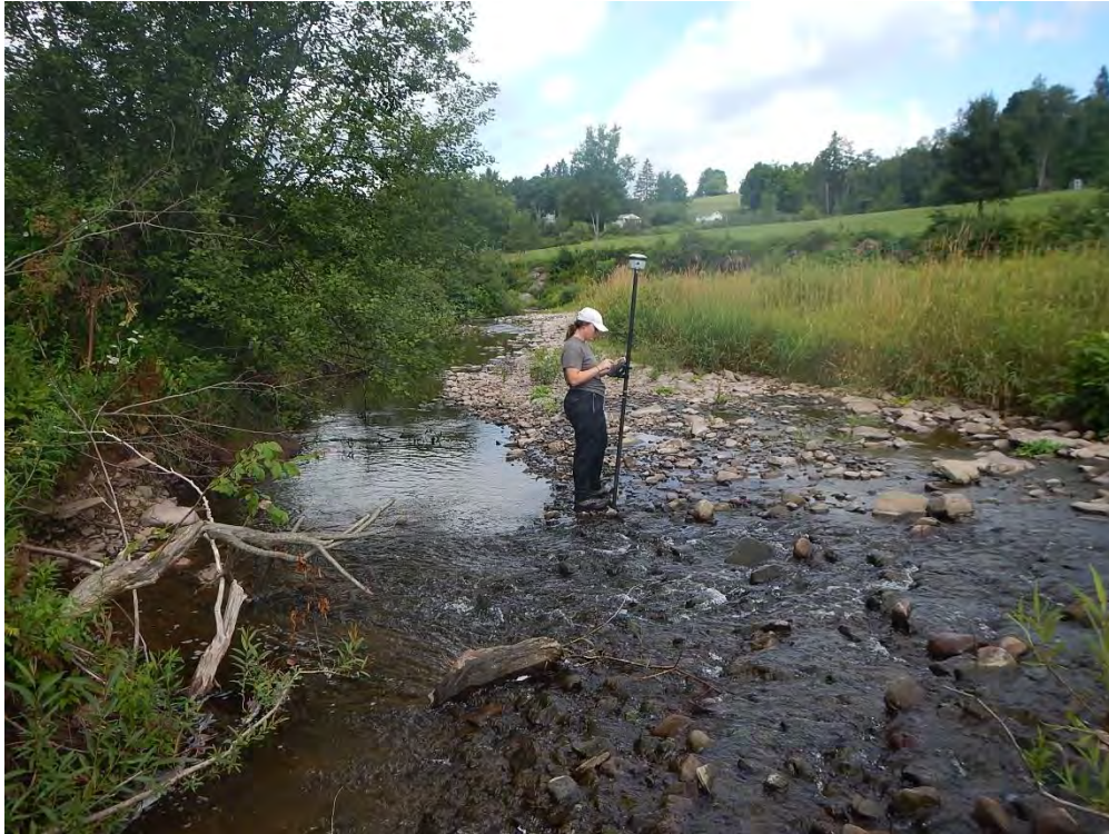
Site 15-a: Transverse bar directing flow into eroding left bank. Photo taken looking downstream at STA ~1060+00.
