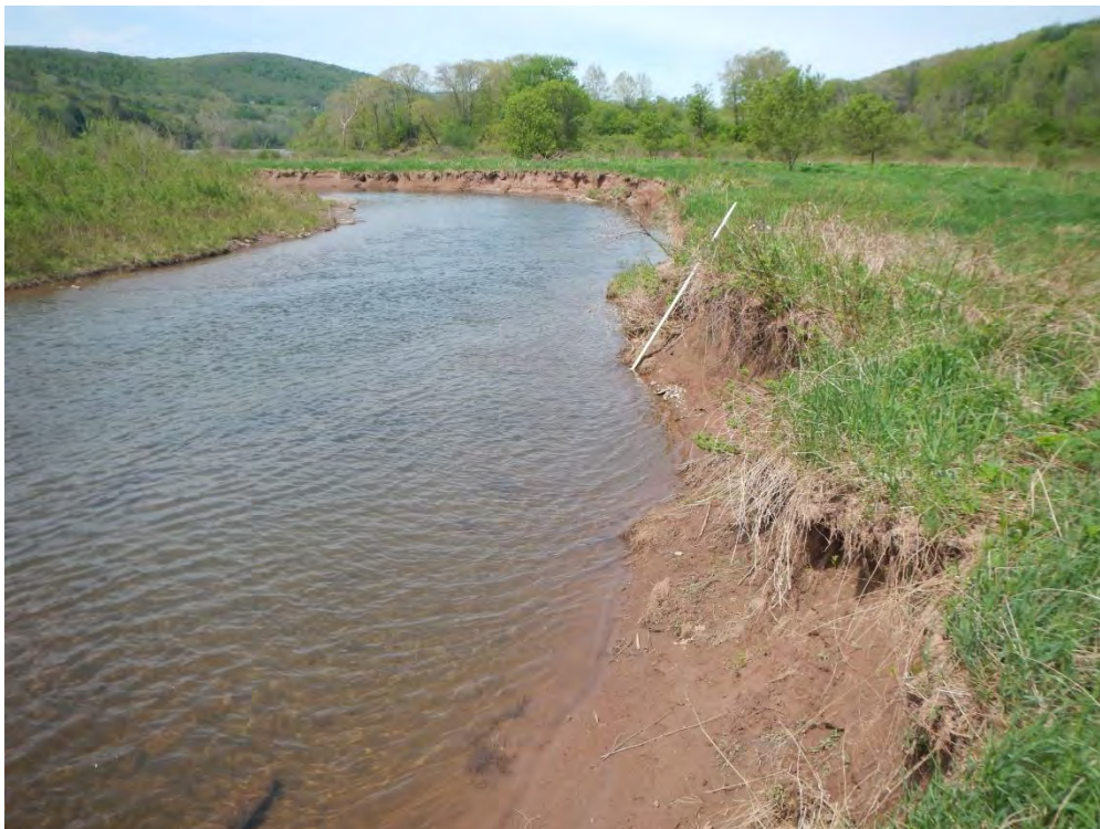
Site 2-a: Erosion along the right bank on a sharp bend. Note the shallow rooting depth and lack of riparian forest buffer. Photo taken looking downstream at STA ~389+00.
