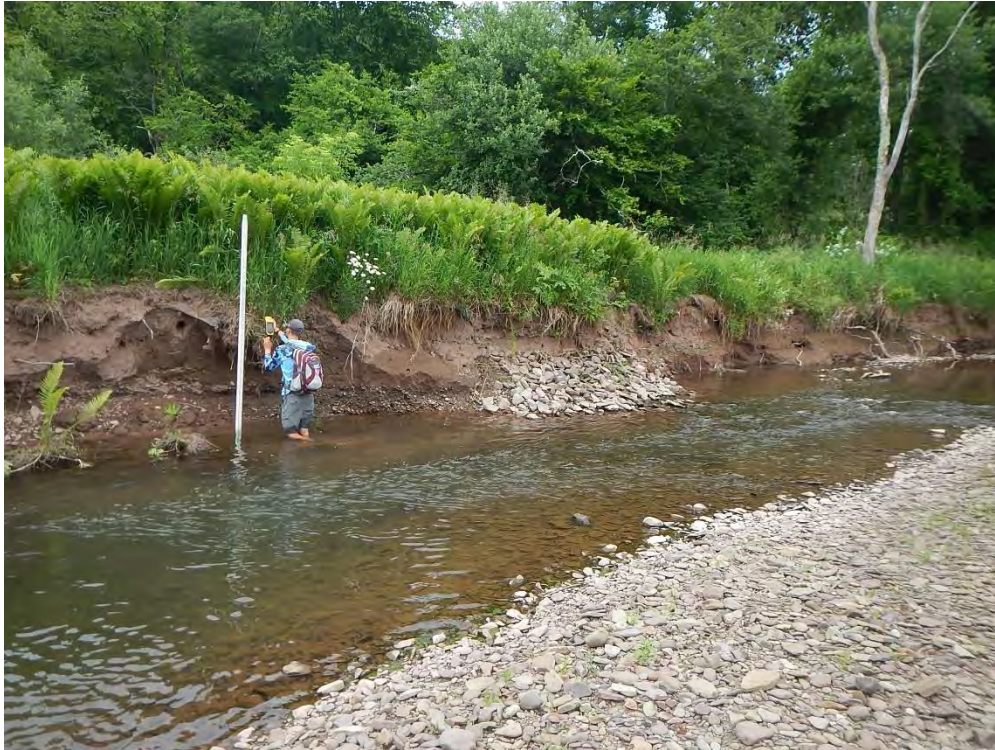
Site 8-b: Erosion along the right bank. Note the shallow rooting depth of the herbaceous vegetation on the bank. Photo taken looking upstream at STA ~706+50.
