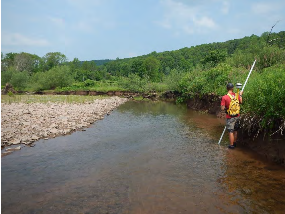
Site 1-b: Erosion along the right bank with an aggrading mid-channel bar along the left bank. Photo taken looking downstream at STA ~383+00.
